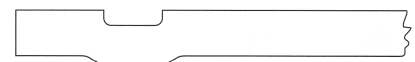
Standard Roll Groove on Standard Weight (S-40) Pipe. (For stainless steel and other IPS pipe)
